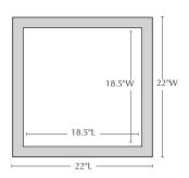
Materials: unsaturated polyester resin, sand, stone powder, talc powder, and fiberglass
